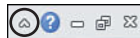
Figure 1.4 Click the arrow by the Help button to minimize the Ribbon. Click it again to make the Ribbon normal again.
